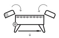
Open the tension locks below the goal boxes, fold them into the playfield and secure them with the bolts. Detach the fixing rod between the legs and take it out.
